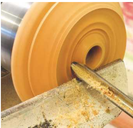
▲ Pic.13 Work the gouge in from the centre and then down from the edge. This is because Les decided to make a small bowl on the base
